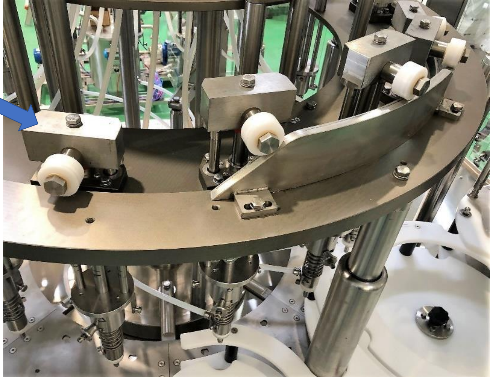
Filling Valve Movement without Piston lifting bottles (Descending Valve system)
