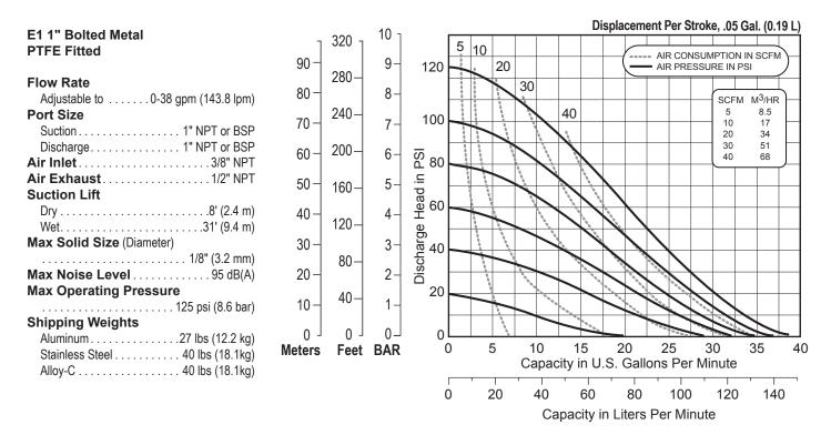
NOTE: Performance based on the following: PTFE fitted pump, flooded suction, water at ambient conditions. The use of other materials and varying hydraulic conditions may result in deviations in excess of 5%.
