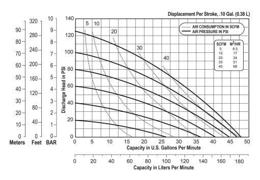
NOTE: Performance based on the following: elastomeric fitted pump, flooded suction, water at ambient conditions. The use of other materials and varying hydraulic conditions may result in deviations in excess of 5%.
