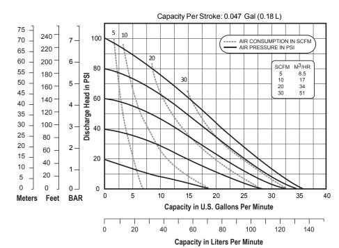
NOTE: Performance based on the following: PTFE fitted pump, flooded suction, water at ambient conditions. The use of other materials and varying hydraulic conditions may result in deviations in excess of 5%.
