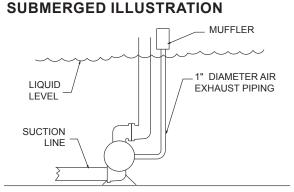
Pump can be submerged if the pump materials of construction are compatible with the liquid being pumped. The air exhaust must be piped above the liquid level. When the pumped product source is at a higher level than the pump (flooded suction condition), pipe the exhaust higher than the product source to prevent siphoning spills.
